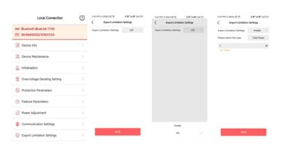
There are two methods to control the export limit, the two methods are alternative to each other. Method1: Export limitation setting is to control the export electricity to the grid. Method 2: Generation limit is to control the electricity generated by the inverter.
