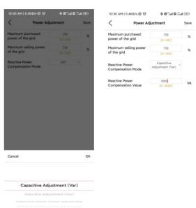
Step 1: Select Inductive Adjustment Var or Capacitive Var according to your local grid regulation. The power range is from -60%Pn.
